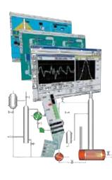
Utilizing the power of PLC it is possible to control the analyzer and also have a local repository of data. This eliminates the use of proprietary data loggers, resulting in a very cost effective, reliable and flexible system architecture, providing easy user interface, data editing and EPA approved report formats.
